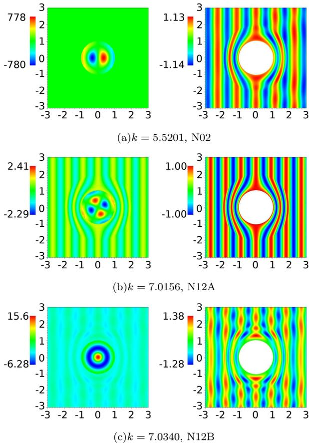
FIG. 4. Snapshots of acoustic pressure fields of the imperfect cloaking with  $\varepsilon = 0.0001$ : total pressure fields on the whole region (left) and outside of the disc  $B_{1.02}$  of radius 1.02 (right)
